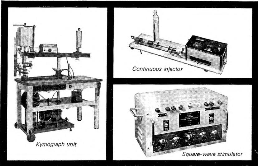
Palmer kymographs such as this are in service in laboratories all over the world, providing smoked paper records of muscle and tissue movement, or through a manometer, of blood pressure. A 6-gear motor gives paper speeds from 1mm to 10mm per second, A.C. time-clock and signal markers and the Starling ventilation pump are fitted.
