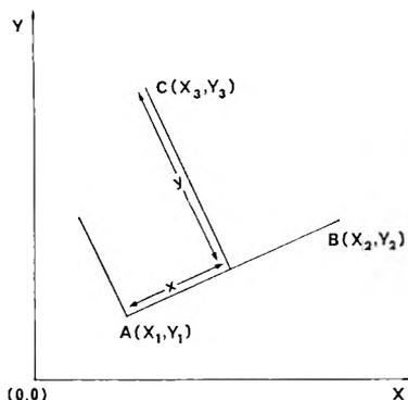
FIG. 2. The transformation of the co-ordinates of a point, C, from those of the reading table to those of the trace.  $X, Y$ , the co-ordinate axes of the reading table.  $AB$ , the baseline of the trace.  $x, y$ , the co-ordinates of the point C relative to the trace.
