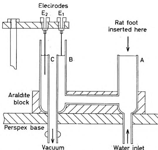
FIG. 1. Glass displacement chamber and electrode assembly.
