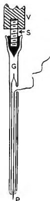
Fig. 6.—Construction of electrodes: V = stem of vibrator, S = screw cemented into electrode, G = glass tubing support for P = platinum wire electrode.
