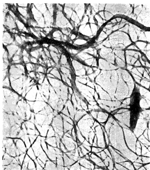
B. Grease after extraction with butylene and ethylene, release of ethylene after heating to 30° C., and reconstitution with oil.
