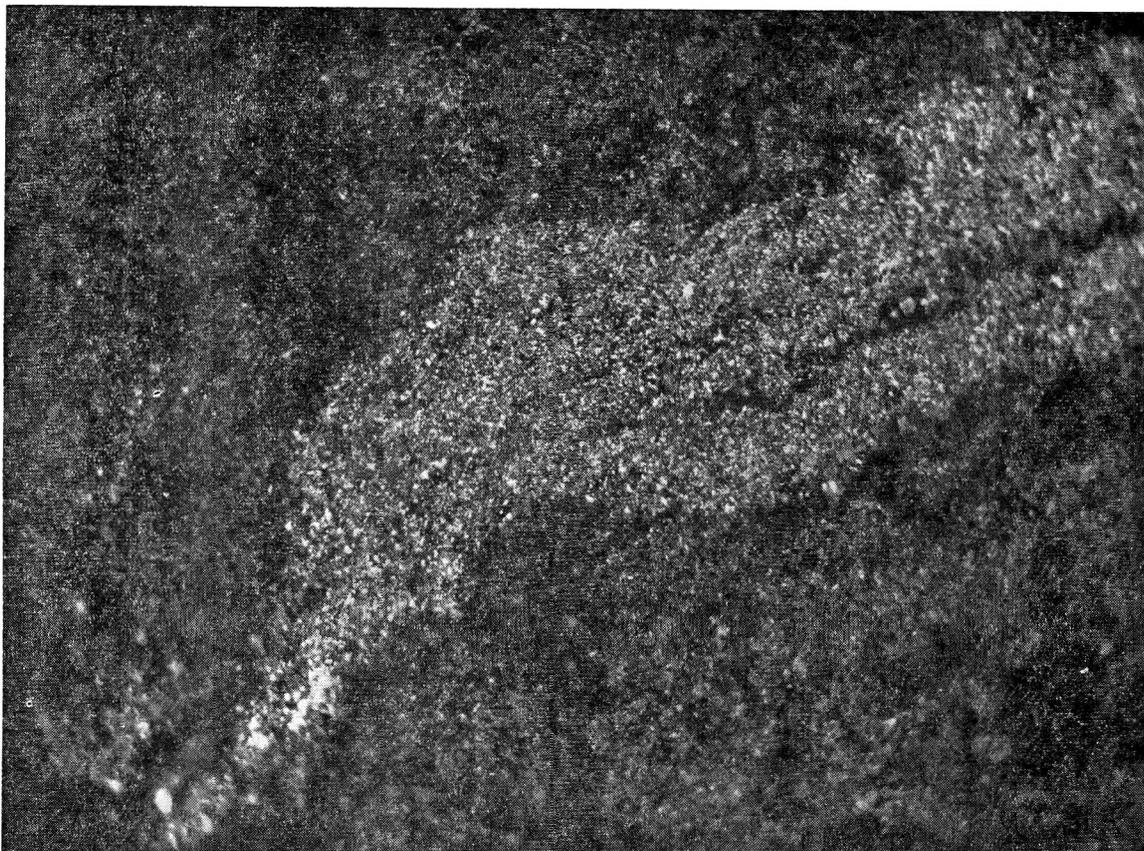
Fig. 1.—Coal-pyrite from Plodder Seam, Lancashire; showing a vein of pyrite in a mosaic of marcasite, magnification 300 $\times$ .
