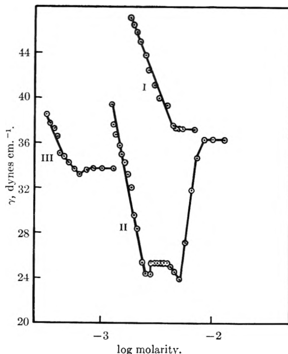
Fig. 1.—Surface tension of p -nonylbenzene sulfonate: I, alone in distilled water at 20°; II, plus 0.5% by weight lauryl alcohol; III, plus 0.5% lauryl alcohol in 0.2 M NaCl
