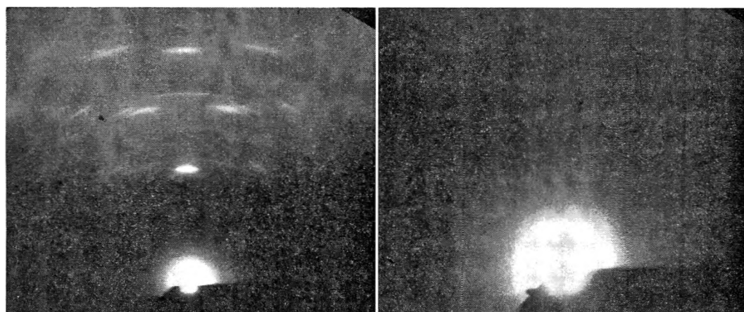
(a) Original silver film deposited in 0.75 mm. N_2 . (b) Same film after heating in air 7 hr., H_2 1 hr., and use for ethylene oxidation for 5 hr.
