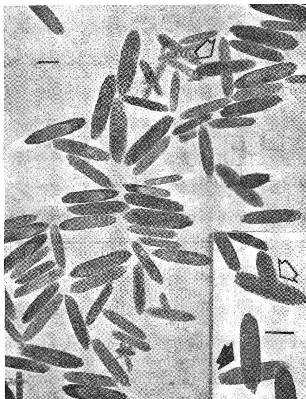
Fig. 1.—Unsectioned, whole crystals of \beta -FeOOH, \times 50,000 , 80 kv. electrons. (In each figure, unless indicated otherwise, the line represents 0.1 \mu .) The insert shows the appearance of a true twin (clear arrow) compared with that of overlapping crystals (solid arrow), \times 77,000 .
