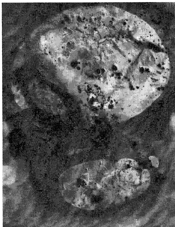
Fig. 1.— \alpha -Lead azide coated with 10.0 atom% of silver. (Chromium shadow transfer replica, magnification 40,000.)
