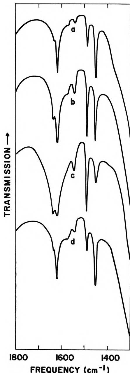
Figure 6. Dual adsorption of pyridine and \text{H}_2\text{O} on silica-alumina: (a) SA exposed to pyridine at 17 mm. and 150^\circ for 1 hr. followed by evacuation at 150^\circ for 16 hr.; (b) exposure to \text{H}_2\text{O} at 15 mm. and 150^\circ for 1 hr. followed by evacuation at 150^\circ for 1 hr.; (c) exposure to \text{H}_2\text{O} at 15 mm. and 25^\circ for 1 hr. followed by evacuation for 1 hr. at 25^\circ ; (d) evacuation for 16 hr. at 150^\circ .
