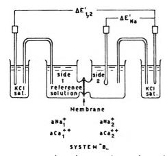
Figure 3. Reference electrode system for membrane titration.
