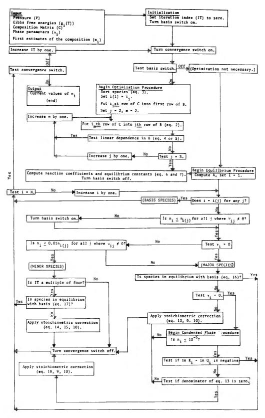
Figure 1. Flow chart for computation procedures.
