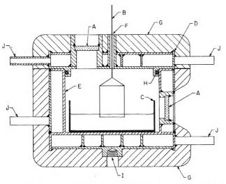
CYLINDRICAL CONSTANT TEMPERATURE CELL FOR A DUNOÜY TENSIOMETER
