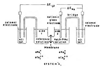
Figure 2. Apparatus for membrane electrode titration.
