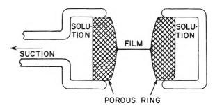
Figure 8. Apparatus for obtaining large hydrostatic suctions within a film produced by withdrawing liquid from a porous ring.
