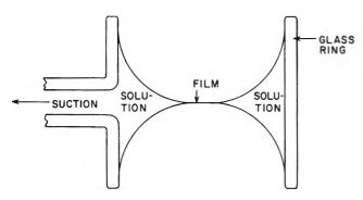
Figure 7. The principle of Scheludko's apparatus for producing films by gradual removal of liquid from a glass ring a few millimeters in diameter.
