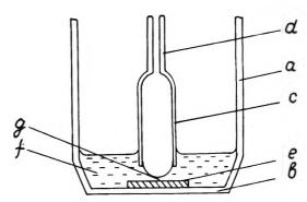
Figure 1. Cell for the investigations of circular liquid films on a solid substrate.
