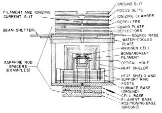
Figure 1. Ion source and furnace arrangement.
