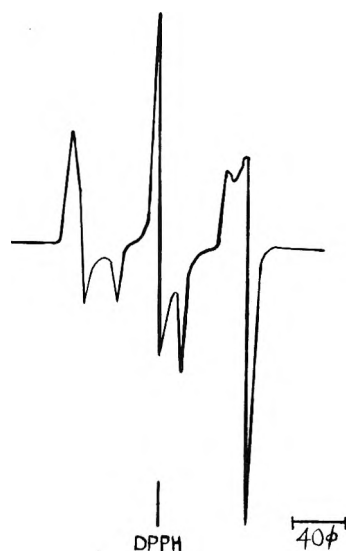
Figure 4. E.p.r. spectrum of photolyzed tetranitromethane at 77°K.
