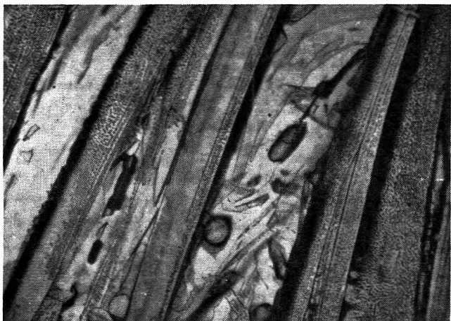
Figure 4. Microstructure of phenanthrene, \times 120 .
