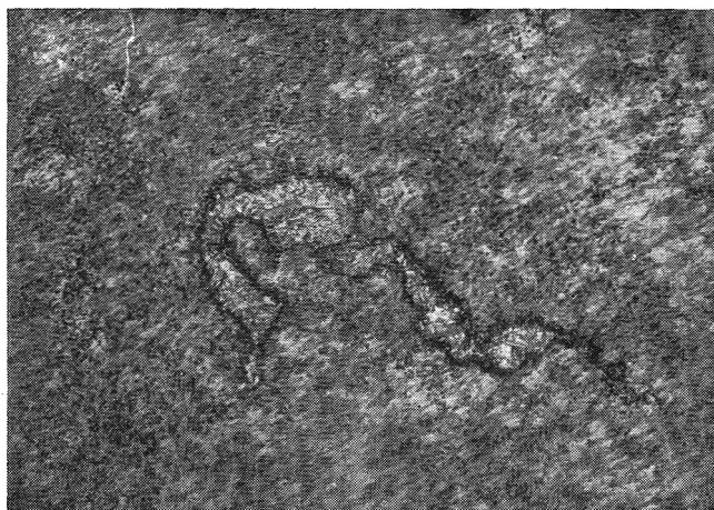
Figure 8. Microstructure of the aged eutectic, \times 120 .
