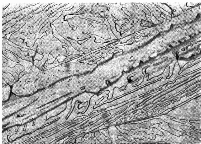
Figure 3. Microstructure of naphthalene, \times 120 .
