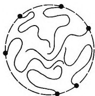
Figure 1. A very schematic representation of the cross section of a spherical micelle. The polar heads are shown on the surface.
