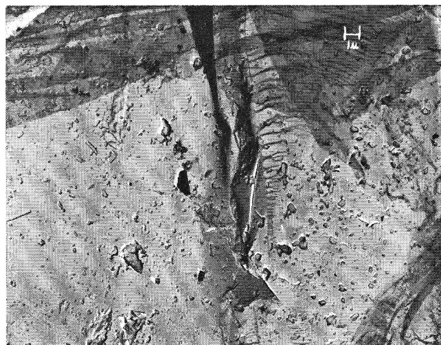
Figure 9. Electron micrograph (13,000 \times ) of surface of a large amorphous silica particle.
