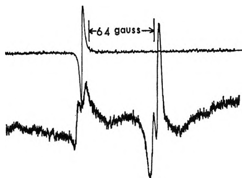
Figure 5. ESR spectrum of zinc oxide outgassed at 500° and treated with methane containing 2% oxygen.
