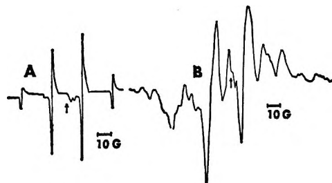
Figure 1. (A) Electron spin resonance spectrum of \gamma -irradiated \text{CH}_3\text{Br} on silica gel at 77^\circ\text{K} ( 3.0 \times 10^{-2} mol fraction); (B) esr spectrum of \gamma -irradiated \text{C}_2\text{H}_5\text{Cl} on silica gel at 77^\circ\text{K} ( 3.6 \times 10^{-2} mol fraction). The arrows indicate g = 2.0028 .
