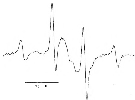
Figure 7. Esr spectrum of radical species produced by reaction of electrons with L -methionine at 77°K. The sharp four-line spectrum is due to the methyl radical. The broad signal in the central portion of the spectrum is most likely the carboxylic dianion.
