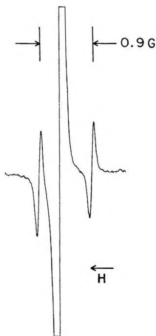
Figure 7. Spectrum during photolysis of an aqueous solution containing 22 g of oxalic acid, 370 ml of isopropyl alcohol, 123 ml of acetone, and 31 ml of concentrated HCl per liter at about 37°. The strongest line is due to reduced oxalic acid. The two weaker lines constitute a 1-1 spectrum due to the reduced monoester of oxalic acid and isopropyl alcohol.
