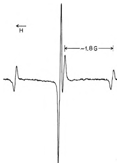
Figure 6. Central part of the spectrum during photolysis of an aqueous solution containing 2.7 g of oxalic acid, 446 ml of ethylene glycol, 115 ml of acetone, and 92 ml of concentrated HCl per liter at about 37°. The strongest line is due to reduced oxalic acid. The 1-2-1 spectrum is due to the reduced monoester of oxalic acid and ethylene glycol.
