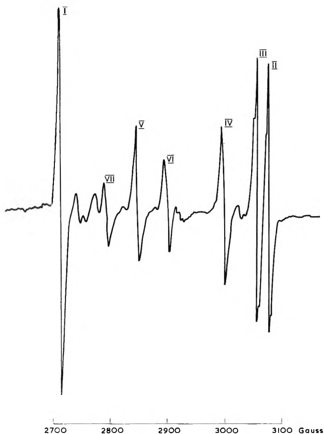
Figure 2. Epr spectrum of X-irradiated nickel acetate at 77°K. Field along b axis.
