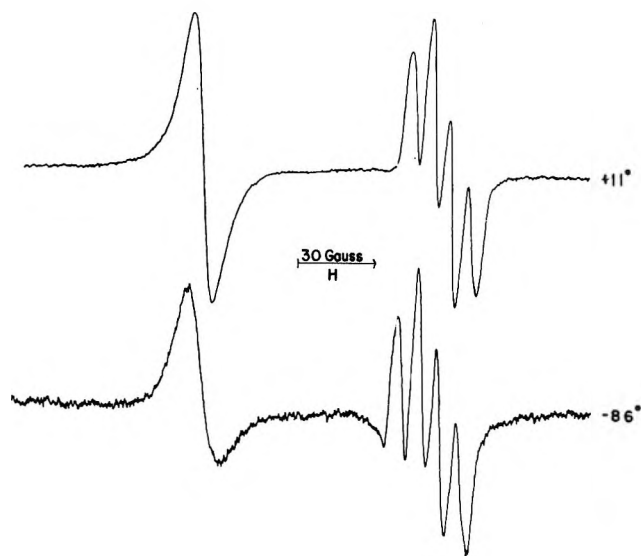
Figure 6. First derivative esr spectra of a 10^{-4} F PTZ-NiTh solution in dichloromethane at +11° (top) and -86° (bottom).
