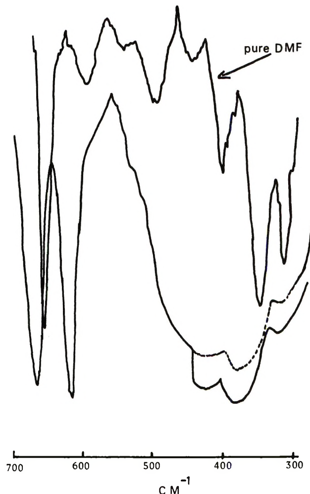
Figure 1. Trace of the ir spectra of pure DMF and a solution of \text{LiClO}_4 in DMF. The vertical line in the spectra at 450 \text{cm}^{-1} is due to a malfunction in the machine. The dotted line more correctly represents the spectrum.
