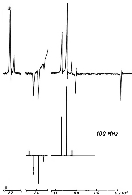
Figure 3. CIDNP during photolysis of BPO in a 1:100 mixture of \text{CH}_3\text{I} and \text{CH}_3\text{COCH}_3 .
