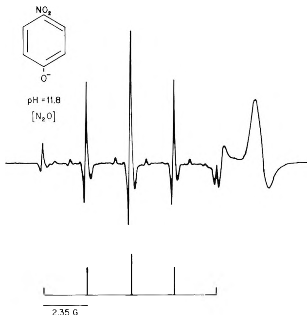
Figure 9. ESR spectrum of p -benzosemiquinone radical ion obtained from an \text{N}_2\text{O} -saturated solution of 10^{-3} M p -nitrophenol at pH 11.8.
