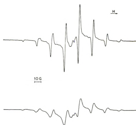
Figure 2. ESR first-derivative spectra of \gamma -irradiated crystalline tert -butyl isothiocyanate recorded under identical spectrometer conditions at 77°K during (upper spectrum) and after (lower spectrum) exposure of the sample to unfiltered tungsten light. These spectra may be compared with those in Figure 1 since they refer to the same sample and the same spectrometer conditions except for a gain setting of 200 in this case instead of 250.
