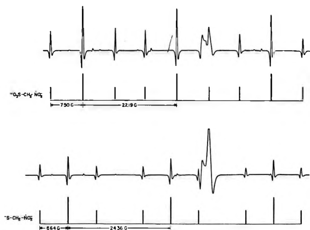
Figure 2. Second-derivative esr spectra of the \cdot\text{SO}_3^- and \cdot\text{S}^- adducts to \text{CH}_2=\text{NO}_2^- . Magnetic field increases to the right. The stick spectra show the lines assigned to the indicated species with the shift in the centers of the patterns corresponding to a difference in g factors of 0.00104. Also present to the right of center is the signal from the silica cell taken at the same gain setting. The values designated as a^N have been corrected for the different second-order shifts and so do not strictly correspond with the separation between the indicated lines. All figures have been made in this same way. Spectra were taken under the conditions [\text{SO}_3^{2-}] = 2 \times 10^{-2} M , [\text{CH}_3\text{NO}_2^-] = 1 \times 10^{-2} M , pH 12.1 and [\text{S}^{2-}] = 2 \times 10^{-2} M , [\text{CH}_3\text{NO}_2] = 1 \times 10^{-3} M , pH 13, respectively. In both cases the solutions were saturated with \text{N}_2\text{O} . Smaller lines are visible in the upper trace for \text{CH}_3\dot{\text{N}}\text{O}_2^- and \text{HOCH}_2\dot{\text{N}}\text{O}_2^- and in the lower trace for -\text{O}_3\text{SCH}_2\dot{\text{N}}\text{O}_2^- .
