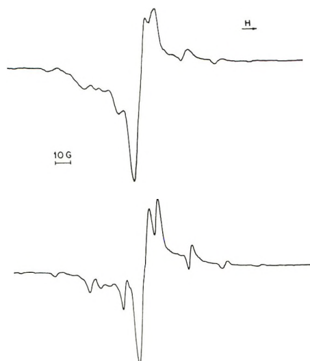
Figure 1. ESR first-derivative spectra of \gamma -irradiated crystalline tert -butyl isothiocyanate recorded under identical spectrometer conditions at 77°K before (upper spectrum) and during (lower spectrum) exposure of the sample to red light (Corning Filter No. 2030). The \gamma -irradiation dose was 0.65 Mrad.
