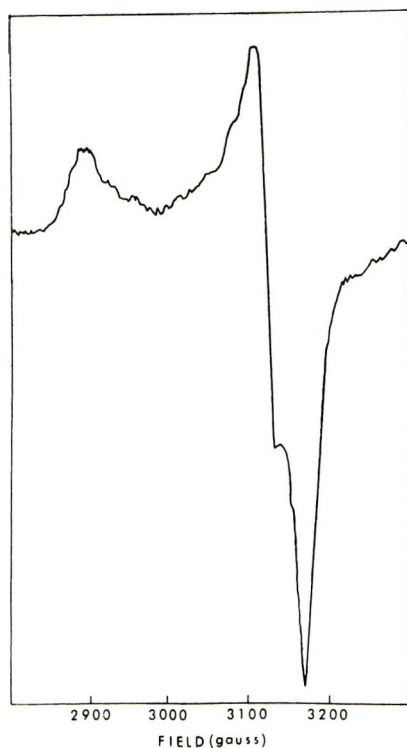
Figure 6. The epr spectrum at room temperature of a powdered sample of \text{Cu}(\text{AEP})_2\text{Br}_2 in the region 2800–3300 G ( \nu = 9.18 GHz).
