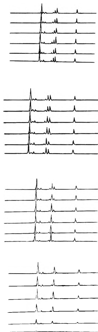
Figure 3. Tracing of TOF experimental record from four sequential photographs for a run at 2700^\circ K . Mass spectra are repeated at 20 \mu sec intervals.
