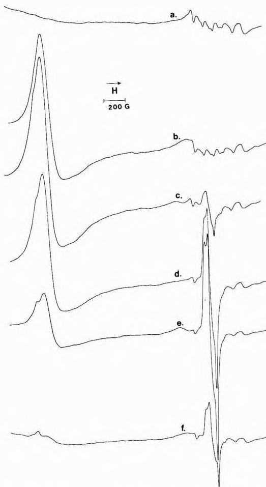
Figure 2. Epr spectra of high-spin and low-spin [\text{Fe}(\text{II})\text{NO}]^{2+} complexes in a Y-type zeolite recorded with the sample at 25^\circ : (a) before addition of NO, amplification of 2; (b) 1 Torr of NO, amplification of 2; (c) 10 Torr of NO, evacuated 15 sec, amplification of 2; (d) sample under vacuum 1 hr at 25^\circ , amplification of 1.2; (e) sample under vacuum 1 hr at 50^\circ , amplification of 1.0; (f) sample under vacuum 1 hr at 100^\circ , amplification of 1.2.
