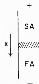
Figure 1. Diagram showing the experimental situation at the time of initial application of an external electric field to a uni-univalent electrolyte diffusion boundary FA-SA. Cross hatching represents the diffuse boundary.
