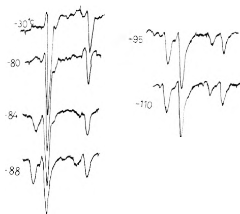
Figure 3. Variation of the spectra with temperature on the hyperfine component of M_1 = -\frac{1}{2} .
