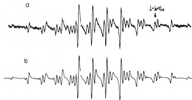
Figure 3. Na-anthraquinone in THF at 44.6^\circ : (a) experimental spectrum; (b) computer-simulated spectrum with k = 2.09 \times 10^6 \text{ sec}^{-1} .
