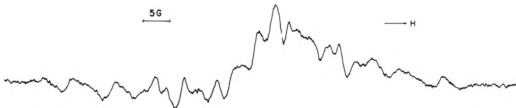
Figure 4. ESR spectrum obtained by irradiation of ethylated glass at room temperature.
