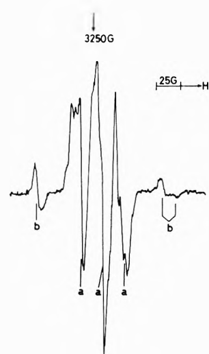
Figure 1. First derivative esr spectra for uv photolyzed \text{Fe}(\text{CN})_6^{3-} in aqueous methanol at 77 K directly after photolysis showing features assigned to \text{H}_2\text{COH} (a) and \text{HCO} (b) radicals.
