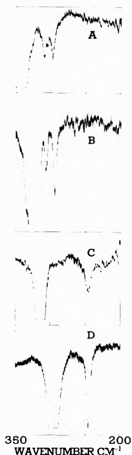
Figure 3. A, B, C, and D, show far-infrared spectra of solid (\text{CH}_3)_3\text{NBH}_3 , (\text{CH}_3)_3\text{NBD}_3 , (\text{CD}_3)_3\text{NBH}_3 , and (\text{CD}_3)_3\text{NBD}_3 , respectively. The ordinate is in arbitrary units of absorption.
