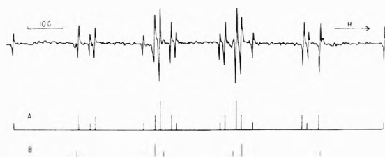
Figure 2. Epr spectrum for the substrate allyl acetate: tp 25°; [\text{TiCl}_3] 0.004 M and [\text{H}_2\text{SO}_4] 0.2 M in the reducing stream; [\text{H}_2\text{O}_2] 0.1 M and [\text{CH}_2=\text{CHCH}_2\text{OOCCH}_3] 0.01 M in the oxidizing stream; total flow rate 3 ml sec -1 equally divided between the two streams. A, First-order stick plot for \text{HO-CH}_2\text{CH}(\text{OH})\text{CH}_2\text{OOCCH}_3 , a triplet (1:2:1) of triplets (1:2:1) of doublets (1:1). B, First-order stick plot for \cdot\text{CH}_2\text{CH}(\text{OH})\text{CH}_2\text{OOCCH}_3 , a triplet (1:2:1) of doublets (1:1).
