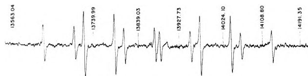
Figure 3. ESR spectrum of the adduct radical \text{Et}_3\text{SiCH}_2\dot{\text{C}}\text{HF} resulting from the reaction of triethylsilyl radical with vinyl fluoride at -45^\circ .
