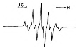
Figure 6. Esr spectrum of a solution of fluoranil in 1 N NaOH containing sodium dithionite, at room temperature.
