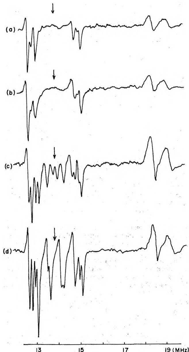
Figure 2. EPR spectra of 9-arylxanthyl radicals: (a) 9-phenyl-, (b) 9- p -tolyl-, (c) 9- o -tolyl-, and 9- \alpha -naphthylxanthyl radical. The free proton frequency is marked with an arrow.
