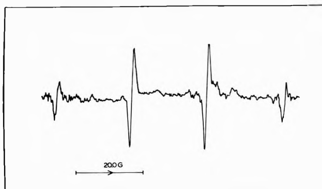
Figure 7. ESR spectrum of the \text{CH}_3 radical formed from the photolysis of 1 \times 10^{-2} M \text{Co}(\text{NH}_3)_5\text{O}_2\text{CCH}_3^{2+} at pH 1 in \text{N}_2 -purged solution. Flow rate of solution through the cell \sim 1 \text{ ml min}^{-1} . The ESR spectrometer (100-kHz modulation frequency) was operated with a modulation amplitude of 1.25 G and a microwave power of 10 mW.
