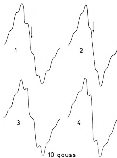
Figure 2. ESR spectra of pyridinyl radicals trapped in alcohol matrices: (1 and 2) P4VP in C 2 H 5 OH and CD 3 OD, respectively ( T = 105^\circ\text{K} ); (3 and 4) computed spectra corresponding respectively to 1 and 2 (see Table III). Vertical arrow g = 2.0032 .
