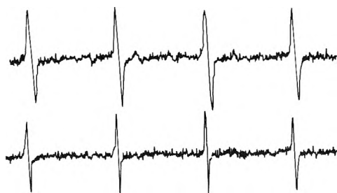
Figure 2. ESR spectra of a solution of K dissolved in pure ethylamine. Upper spectrum was taken with peak-to-peak modulation amplitude, 2h_m = 0.8 G , while for the lower spectrum 2h_m = 0.2 G . In the upper spectrum, a weak central line due to the solvated electron is barely perceptible, while in the lower spectrum no central component can be detected. The upper spectrum also shows some weak lines due to the ^{41}K ( \sim 7\% natural abundance) monomer.
