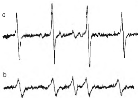
Figure 1. (a) ESR spectrum of a solution of K dissolved in ethylamine containing approximately 15% by volume methylamine. The concentration of monomer is 1.4 \times 10^{-6} M . The central component due to the solvated electron, as well as weak lines due to ^{41}K monomers, is clearly in evidence here. (b) Same at somewhat lower concentration. At this lower concentration, the central component due to the solvated electron is essentially equal in amplitude to the monomer lines.
