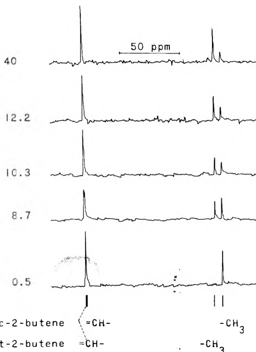
Figure 2. ^{13}\text{C} spectra monitoring cis -2- \text{C}_4\text{H}_8 isomerization on \text{Al}_2\text{O}_3 -B degassed at 250 °C. Numbers on left indicate time in hours elapsed since sample preparation.
