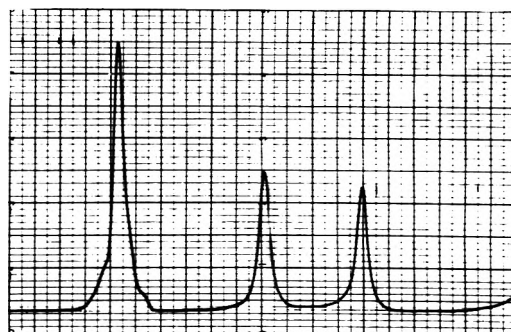
Figure 3. Spectrum of liquid \text{CCl}_4 in the sample cell: spectral resolution 5\text{ cm}^{-1} ; scan speed 25\text{ cm}^{-1}/\text{min} ; photon counting level 1 \times 10^6\text{ Hz} ; period 5.
