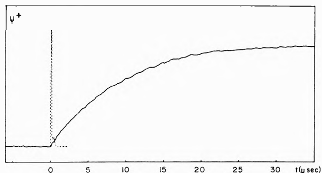
Figure 3. Detail of the radical ion current growth kinetics, average of 32 pulses. The dotted curve is the single-shot response of the instrument to a delta function current input (10-ns laser flash, detected by p-i-n photodiode, response 1 ns).
