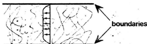
Figure 2. Flow regime of a polyelectrolyte solution in a tube.
