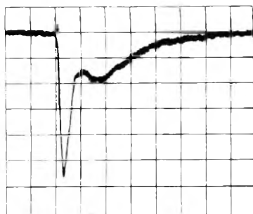
Figure 1. Emission vs. time at 725 nm ( 2p_{10} \rightarrow 1s_4 ) in 840 Torr of Ne. The time scale is 100 ns/division. The arrow indicates the end of the approximately 5-ns wide electron pulse.
