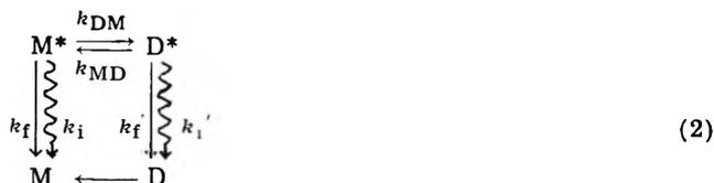
where  $M^*$  is the LE state,  $D^*$  the intramolecular excimer state,  $M$  the ground state of the anti form of mePy, and  $D$  the ground state of the syn form of mePy. In eq 2,  $k_f$  represents the radiative rate constant of LE fluorescence and  $k_i$  the radiationless rate constant,  $k_f'$  and  $k_i'$  represent those of excimer, respectively.
