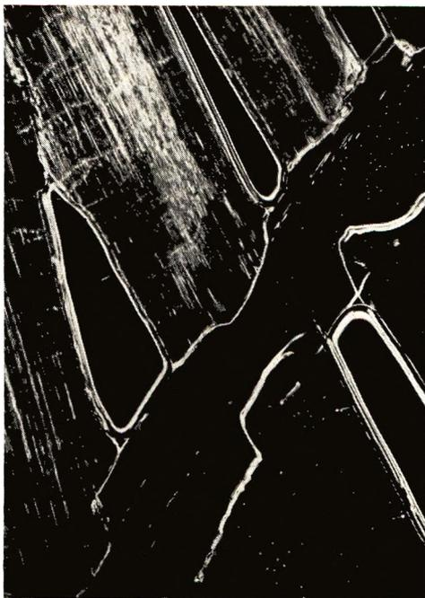
Fig. 4. Polyoxymethylene produced from trioxane at  $54^{\circ}\text{C}$ . Magnification  $100\times$ .
