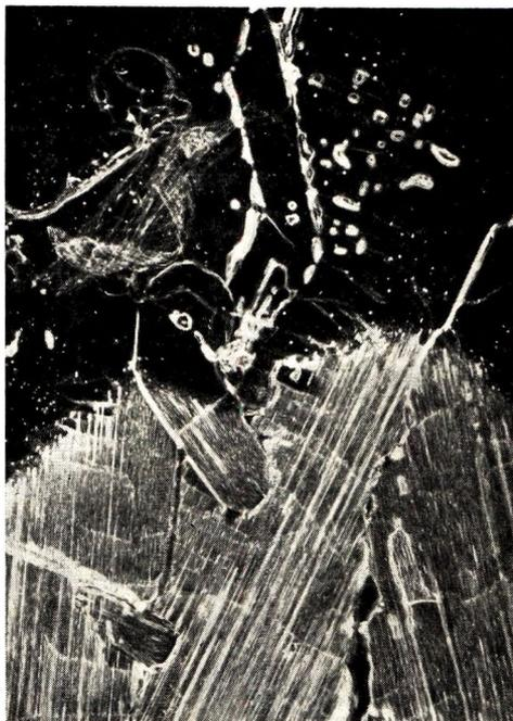
Fig. 5. Polyoxymethylene produced from trioxane at 54°C. Magnification 100 $\times$ .
