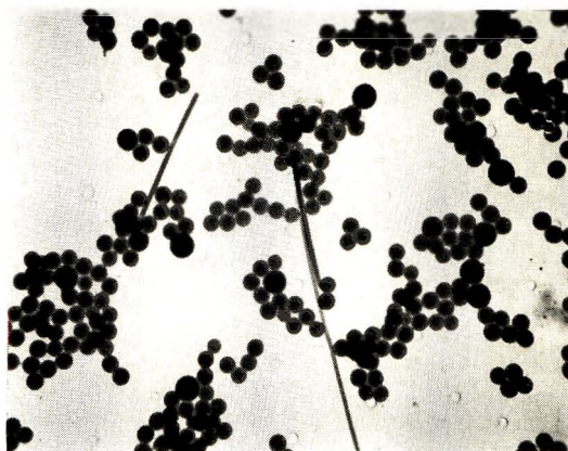
Fig. 3. Sample B-5. Particle diameters: sample = 1335 A., standard = 1880 A. 19,500 \times .
