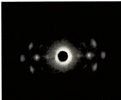
Fig. 3. X-Ray diagram of a wholly aromatic ordered copolyamide fiber (III, Table IV).
