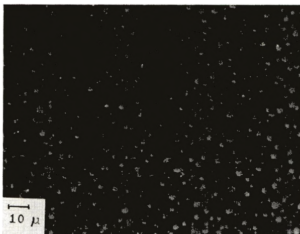
Fig. 1. Rubber particles (white) in a continuous phase of polystyrene (black), prepared by polymerization of a solution of polybutadiene rubber in styrene with agitation (final polymer).
