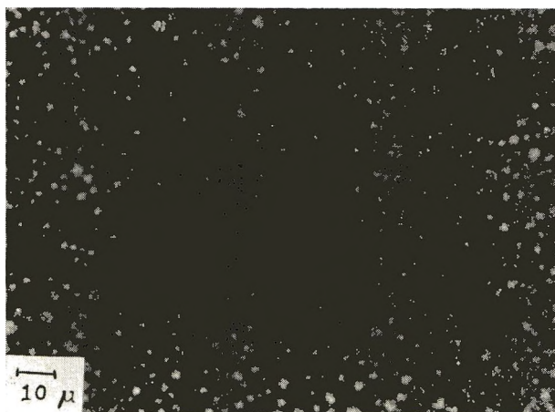
Fig. 6. POO-emulsion after the phase-inversion point in the polymerization of a solution of polybutadiene rubber in styrene.
