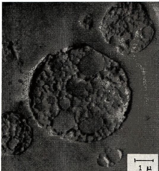
Fig. 8. Electronphotomicrograph of type I and type II occlusions of polystyrene in rubber particles; final polymer formed by polymerization of a solution of polybutadiene rubber in styrene.
