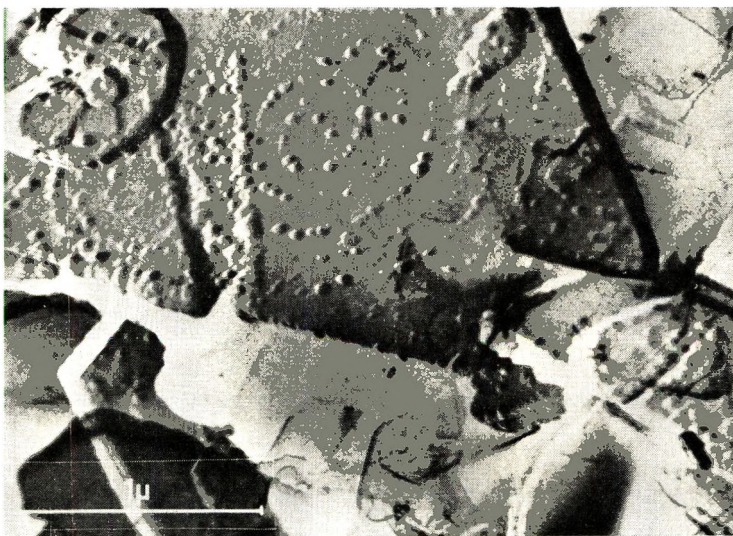
Fig. 6. \alpha - \text{TiCl}_3 crystals, after reaction with \text{AlMe}_3 and polymerization of propylene. 50,000 \times . Carbon replica.
