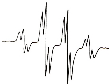
Fig. 1. ESR spectrum obtained during autoxidation of PPH containing AH early stage of reaction.
